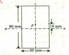
The maximum bending stress produced in the bar at xx is nearly
